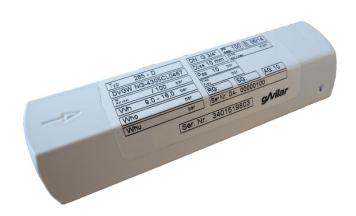
The 285 D relief valve is installed downstream of pressure regulators to relieve limited volumes of gas. This valve may be used where venting to the atmosphere is acceptable and some pressure relieving tolerance is acceptable.
