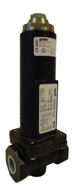
The 155 D relief valve is installed downstream of pressure regulators to relieve limited volumes of gas. Used where venting to the atmosphere is acceptable, it provides a cost- effective solution to prevent safety shut-off valves from triggering in case of creep leaks from regulators. This valve is ideal for medium pressure settings and offers a wide setting range and robust performance.
